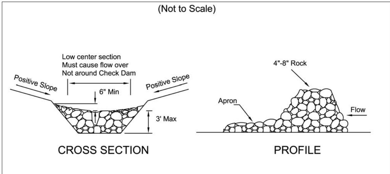
1. The check dam shall be constructed of 4-8 inch diameter stone, placed so that it completely covers the width of the channel. ODOT Type D stone is acceptable, but should be underlain with a gravel filter consisting of ODOT No. 3 or 4 or suitable filter fabric.
