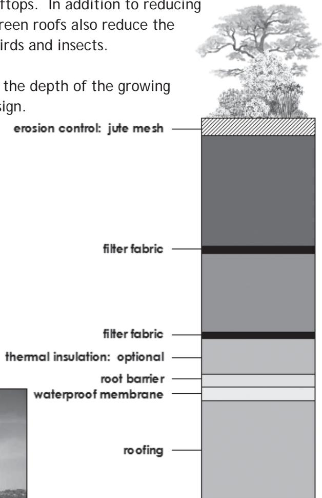
**NOTE:** A detailed structural analysis of the existing building is required to ensure it can adequately support the weight of a vegetated rooftop, before one can be constructed.
