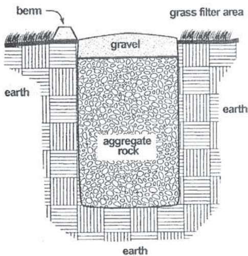
Infiltration trenches are classified in two ways:
