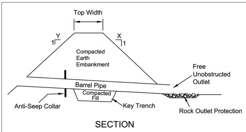
Figure 6.1.6 Embankment Design
