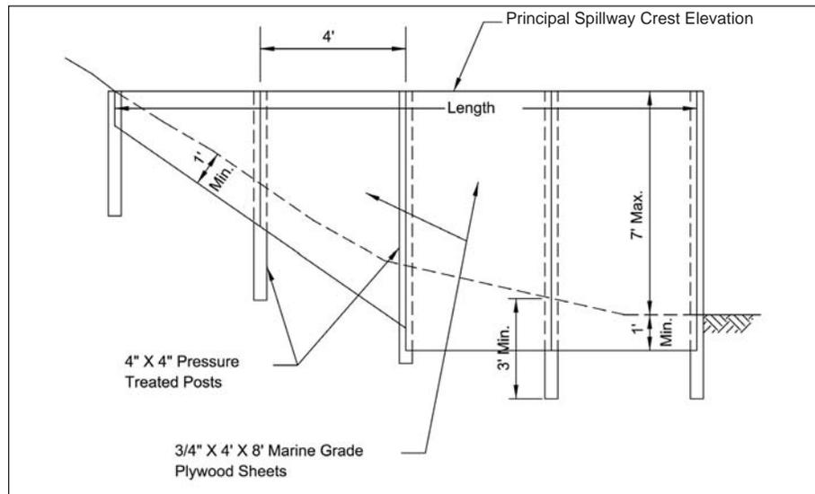
Figure 6.1.4 Typical construction of a solid baffle
