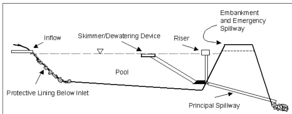
Figure 6.1.2 Typical components of a settling basin
